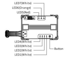
①LED1, LED2, LED3, LED4 are white lights and show the battery SOC and lifespan
