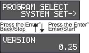
From the main charge menu press the +/- button to switch to the "PROGRAM SELECT SYSTEM SET" position
